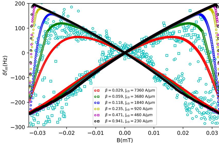
FIG. S3. Plot of the mechanical frequency shift with the magnetic field for different combinations of  $J_{c0}$  and  $\beta$ . Data with circle and square markers represent forward and reverse magnetic sweep, respectively.
