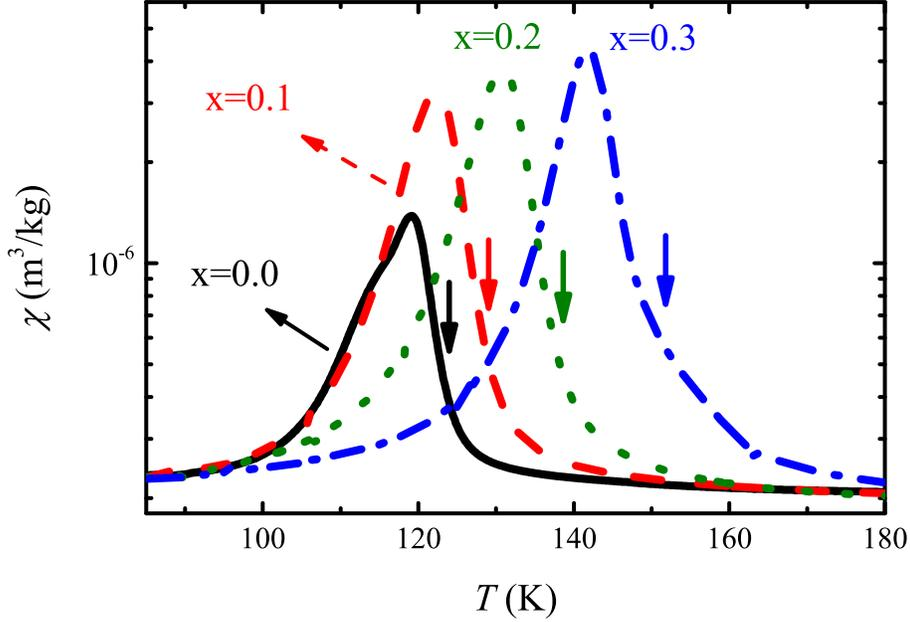
**Figure D1.** *ac*-Magnetic susceptibility curves for  $\text{Ca}_{2-x}\text{Y}_x\text{MnReO}_6$  with  $x=0.0$ , 0.1, 0.2, and 0.3. The estimated magnetic ordering transition temperatures are indicated by vertical arrows.
