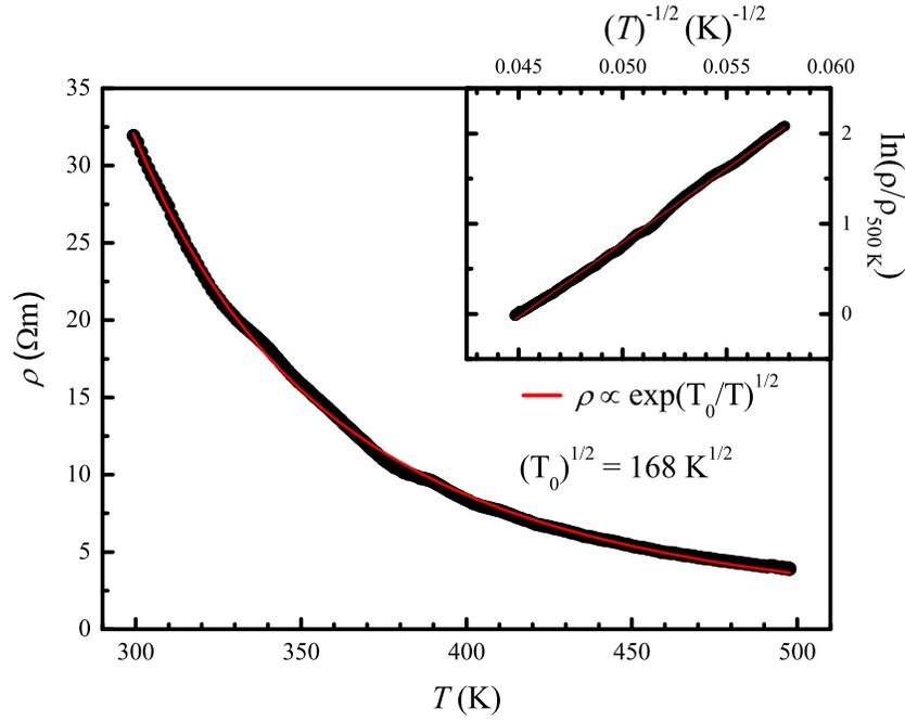
**Figure E1.** Resistivity as a function of temperature for CYMRO (sample 2) with an exponential fitting (red line) for a  $\rho \propto \exp(T_0/T)^{1/2}$  function (ES-VRH model, see text). The inset panel shows the plot of  $\ln(\rho/\rho_{500\text{K}})$  versus  $T^{-1/2}$ , where  $\rho_{500\text{K}}$  is the resistivity measured at 500 K.
