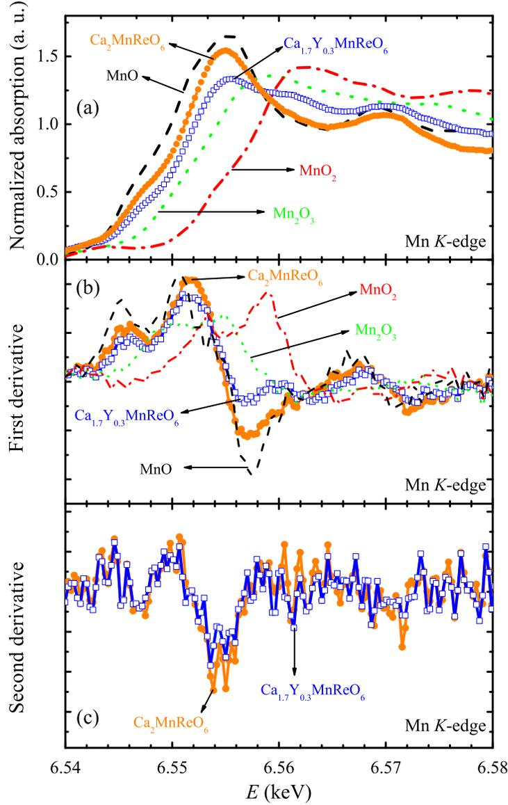
**Figure 5.** (a) X-ray Absorption Near Edge Structure (XANES) at the Mn  $K$  edge of CMRO (closed circles), CYMRO (open circles), and the reference materials MnO (dashed line),  $Mn_2O_3$  (dotted line),  $MnO_2$  (dash-dotted line) and metallic Mn (solid line). (b) First and (c) second derivatives XANES spectrum of CMRO and CYMRO at the Mn  $K$  edge.
