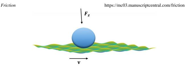
Fig. 1 A spherical tip on a fluctuating surface is squeezed by a normal load  $F_z$  while moving with the velocity of **v**. The fluctuations are described by a cosine wave function and approximated further to the first two terms. The quantization in Sec. 3 is about the surface fluctuations but not the sliding spherical particle. That is, the spherical deformable particle is made up of thousands of atoms with negligible quantum effects like tunneling or delocalization in the wave function.
