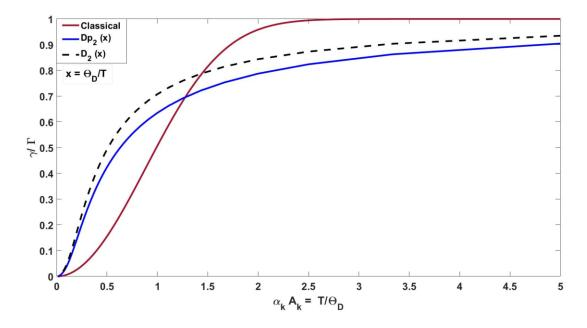
Fig. S1 A comparison between the classical (red) and quantized (blue) kinetic friction coefficients by assuming  $(\alpha_k A_k)_{\text{max}} = T / \Theta_D$ . The dashed line is the second Debye function, Eq. (46), as the first approximation of the quantized friction coefficient. The blue line is Eq. (49), and the red line is the classical Eq. (21) including unsaturated cases.
