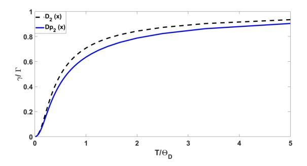
Fig. 2 Kinetic friction coefficient as a function of temperature for the quantized force of Eq. (40). The asymptotic value  $\Gamma$  is identical to the classical case (Eq. (23)). The dashed line refers to the second Debye function  $D_2(x)$ ; an approximation by the quantized amplitudes but classical phases (Eq. (46)). The blue line  $Dp_2(x)$  has counted for both quantized amplitudes and phases in Eq. (49).
