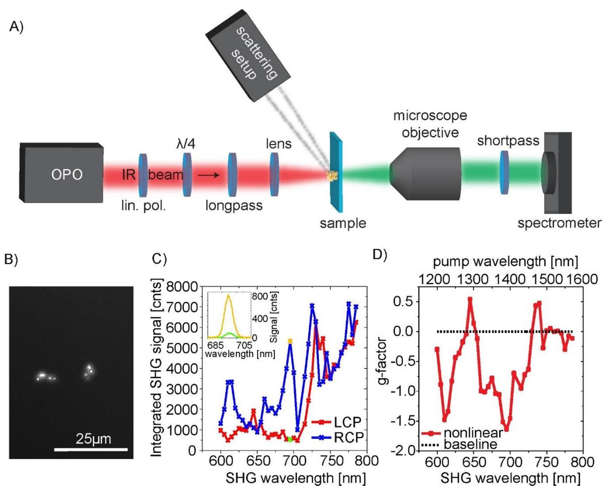
**Figure 4: Results for the nonlinear g-factor.** (A) A coherent laser beam, generated by an OPO, initially passes the polarization optics for generating the circular polarization input and a subsequent long pass to filter any non-infrared light. A lens focuses the beam onto the NP and the generated SHG is collected by a microscope objective. The SHG is separated from the NIR wavelengths by a short pass filter and
