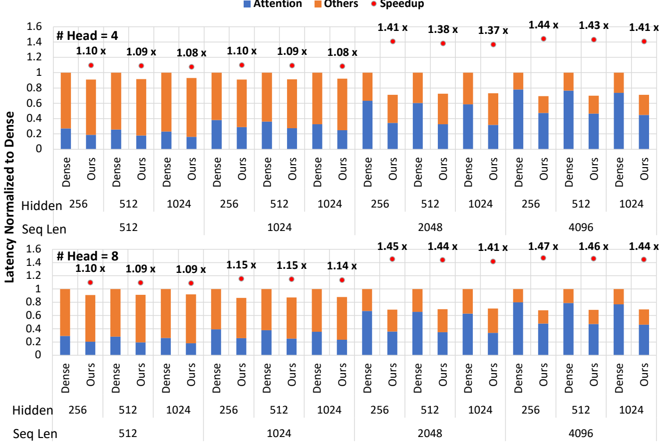
Figure 15: End-to-end inference latency break down under bfloat16.
