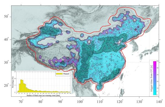
**Figure 3.** Maps showing the estimated EEW system trigger time  $T_{tri}$  from the earthquake origin time for the planned network assuming data transmission latency of 1 s. The areas colored in cyan have the fastest system trigger. The histogram in the bottom left shows the binned distribution of the blind zone radii inside Mainland China obtained from Equation (1) by multiplying it by  $V_S = 3.5$  km/s. Same as Figure 1.
