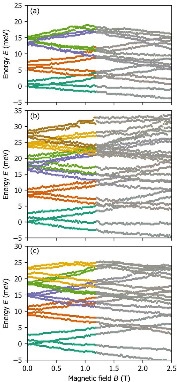
FIG. 12. Experimental data as obtained from the transport measurements on three quantum dot systems QD1, QD2, and QD3. (a) Single-particle energy lines as a function of perpendicular magnetic field  $B$  for QD1 system. Panels (b) and (c) show the same quantity for QD2 and QD3, respectively. The line coloring corresponds to the averaged energy lines displayed in Fig. 6. Gray-colored data above  $B = 1.2$  T are not used in our fitting.
