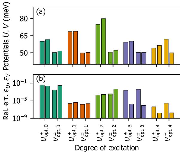
FIG. 7. Values (a) and statistical errors (b) of confining  $U$  and gapping  $V$  potentials for QD3 based on the HRS (and CRS-LM) for the lowest-lying energy pair  $i = 0$  optimization routine. Notation  $Q_{\text{opt},i}^{\pm}$  comprises potential  $Q \in \{U, V\}$  of increasing (+) and decreasing (-) spectral line from  $i$ -th spectral couple consisting of degenerated states at  $B = 0$  T.
