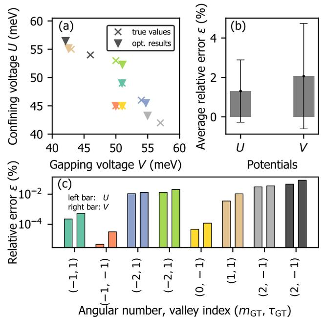
FIG. 13. Testing of the CRS-LM algorithm on the numerically generated target states from Hamiltonian (1). (a) Target states (crosses) and computed continuous parameters (triangles) in the  $U - V$  plane. (b) Relative average error of the associated continuous parameters  $U$  and  $V$ . Panel (c) depicts how the relative errors are distributed among the discrete quantum numbers of the respective target state.
