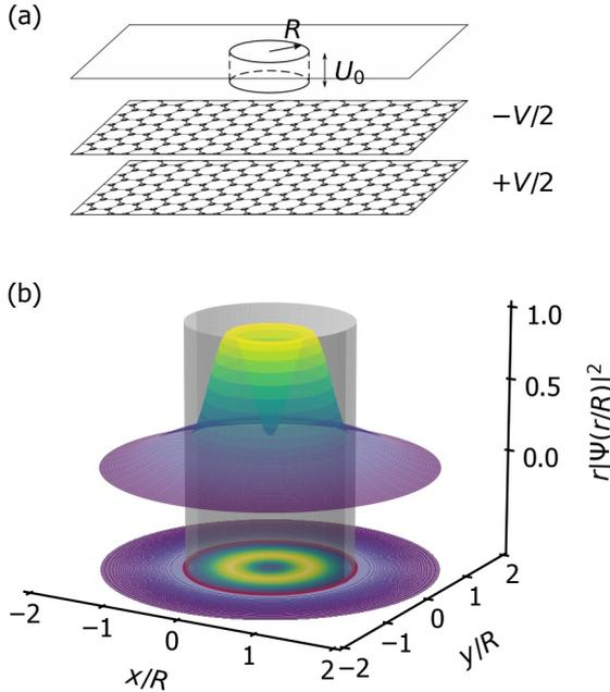
FIG. 1. (a) Illustration of confining potential  $U$  [ $U_0 = U(R)$ ] and gapping potential  $V$  for a quantum dot realized in a bilayer graphene; (b) Visualization of the bound state wavefunction for  $m = 0, \tau = 1, U = 60$  meV,  $V = 50$  meV (top). The projection of the wavefunction is shown in the bottom part of the plot with the gray cylinder indicating the edge of the quantum dot. The red circle indicates the edge of the quantum dot in the projected plane.
