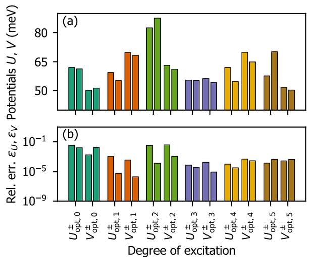
FIG. 15. Fitted values (a) and associated statistical errors (b) of confining  $U$  and gapping  $V$  potentials for QD2 as a result of the application of the HRS (CRS-LM) optimization routine.  $Q_{\text{opt},i}^{\pm}$  denotes the potential  $Q \in \{U, V\}$  of the increasing (+) and decreasing (-) spectral line from the  $i$ -th spectral couple consisting of degenerated states at  $B = 0$  T.
