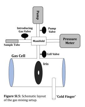
the exact pressure required in the manifold in order to achieve the desired pressure in the gas cell. By opening the cell valve we let the reporter gas condensate at the 'cold finger' until the pressure gauge reads '0' (namely <<0.1torr in our case). We close the cell valve and remove the liquid nitrogen from the cold finger, allowing it to thermalize and the gasses to homogeneously evaporate in the closed gas cell.
