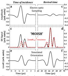
**Figure 1:** THz-induced orientation of 10torr Methyl-Iodide (CH<sub>3</sub>I) at room temperature. (a) Electro-optic sampling signal. (b) Second harmonic (MOISH) signal (probe intensity $1.1 \cdot 10^{14}$ W/cm<sup>2</sup>). (c) Simulated orientation dynamics.
