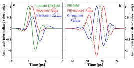
**Figure 3:** Simulation of the different  $\chi^{(2)}$  contributions at (a) t=0 and (b) t=T<sub>rev</sub>. The green curve depicts the incident THz field resulting in electronic (red curve) and the nuclear orientation (blue curve) contributions to the nonlinear susceptibility  $\chi^{(2)}$ .
