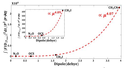
Figure SI.4: Extrapolated collision-free FID energy vs. the molecular dipole, showing  $\propto \mu^4$  power law dependence.
