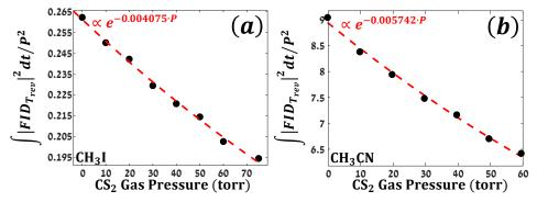
**Figure SI.6ab:** Figures a and b depict the EOS measurements done in gas-mixture of 10torr  $CH_3I/12torr CH_3CN$  and with varying  $CS_2$  pressures respectively.
