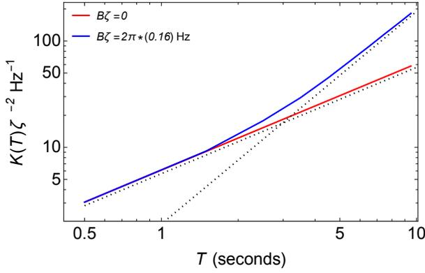
FIG. 1: IQFI ( $K(T)$ ) for using  $X_{\pi/2}$  pulses. Depending on the magnetic field strength we observe a more rapid accumulation of IQFI. The dashed lines are  $\sim T$  and  $\sim T^2$  scalings to guide the eye. For non-zero magnetic field, we see that a crossover from quadratic to linear scaling occurs when  $BT\zeta \ll 1$  (where the perturbative results are valid).
