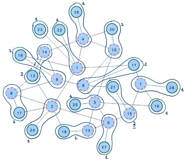
FIG. 7. Graph of the random network with  $N = 28$  here investigated and extracted from Ref. 51. Nodes are grouped by pairs (13) except nodes 19 and 23 which are left unpaired. Nodes encircled in green are sensors and those with red dashed contours are not. The rank  $l$  of the layer for constructing the observer is also reported.
