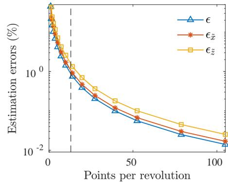
FIG. 3. Estimation errors —  $\epsilon_{\tilde{x}}$  and  $\epsilon_{\tilde{z}}$  — as a function of the number of points per revolution. The Nyquist criterion returns at least 13 points per revolution to avoid undersampling effect.
