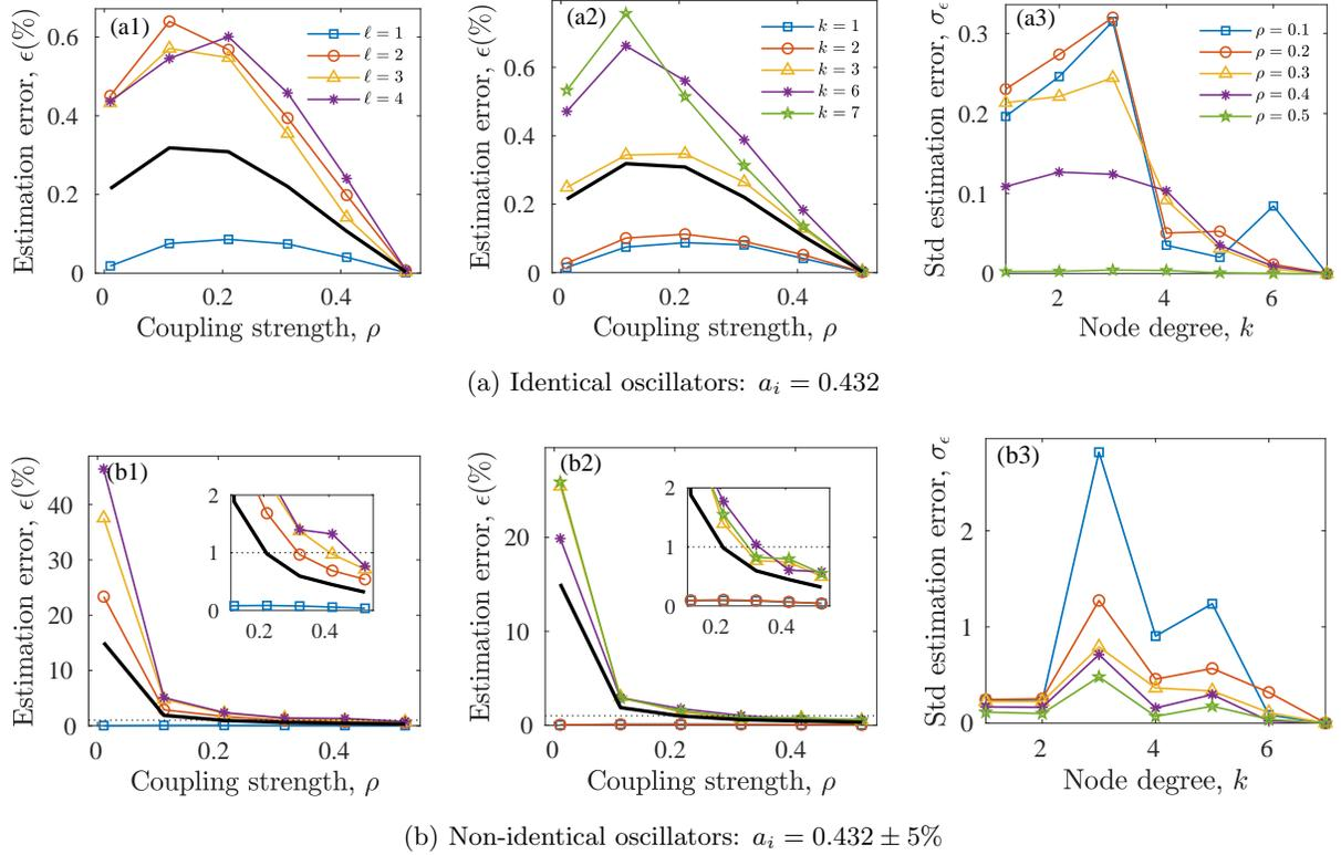
FIG. 10. Dependence of the estimation error  $\epsilon$  on the reconstruction layer  $l$  [(a1) and (b1)] and on the node degree  $k$  [(a2) and (b2)] as a function of the coupling strength for the small network investigated in Fig. 9. The standard deviation of the estimation error within each node degree  $k$  is shown for several coupling values in (a3) and (b3). Legends on top panels apply to the bottom ones. Insets are blow ups of the main plot. Black curves show average quantities.
