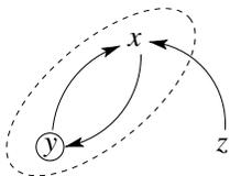
FIG. 1. Pruned fluence graph of the Rössler system where an edge is drawn between  $i$  and  $j$  nodes (variables  $x$ ,  $y$ , and  $z$ ) whenever  $J_{ij}$  in Eq. (10) is a nonzero constant. A dashed oval surrounds the root strongly connected component (rSCC). Edges  $i \rightarrow i$  (self-loops) are omitted since they do not contribute to the determination of the rSCC. Variable  $y$  is encircled as it provides global observability of the system.
