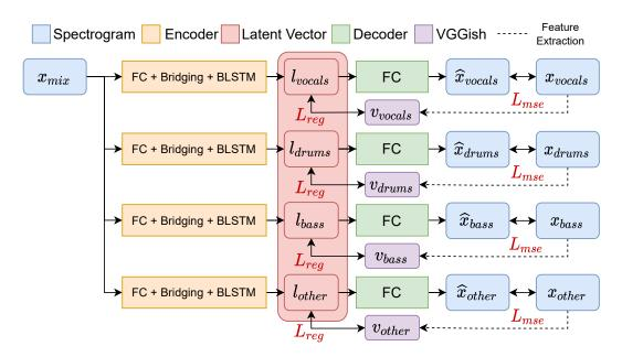
Figure 1: Overview of the X-UMX structure and our proposed training pipeline for the two proposed regularization methods.  $\hat{x}$  denotes the estimated target spectrograms; x denotes the ground truth spectrograms; t denotes the latent vectors; t denotes the VGGish features; t denotes the Mean Square Error and Regularization loss respectively. FC denotes fully-connected layers. The dotted line represents the feature extraction process by VGGish.
