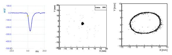
Figure 3: (Left) typical amplified signal from the DL anode; (middle) 2D image of the focused electrons (RF is OFF); (right) 2D image of the scanned electrons (RF is ON).
