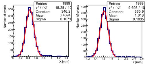
Figure 4: Distribution of X and Y coordinates of anode hit positions (RF is OFF), produced by the AREAL pulsed laser beam.
