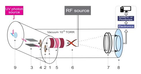
Figure 1: Schematic of the RF timing technique. 1-Tantalum disc cathode; 2-accelerating electrode; 3-permanent magnet; 4-collimator; 5-electrostatic lens; 6-helical RF deflector; 7-dual chevron-type MCP; 8-delay-line anode; 9-UV photon transmission window.
