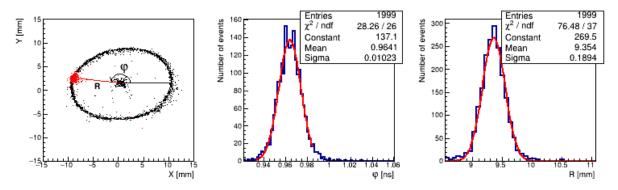
Figure 5: (Left) 2D image of anode hit positions; (middle) distribution of phase; (right) distribution of radius of the scanned electrons.
