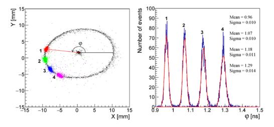
Figure 6: (Left) 2D images of anode hit positions; (right) phase distributions of the 500 MHz scanned synchronized photoelectrons. The different phases are labeled 1 - 4.
