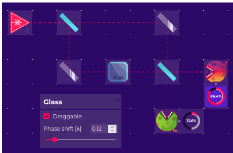
Fig 15 Changing relative optical paths in the Mach-Zehnder interferometer. We use the high-intensity visualization mode.
