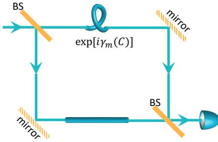
FIG. 4. Detection of the geometric phase  $\gamma_m(C)$  for twisting photons carrying orbital angular momentum via Mach-Zehnder interference. In experiments, an extra Dove prism will be added in the lower optical path after the first beam splitter (BS).
