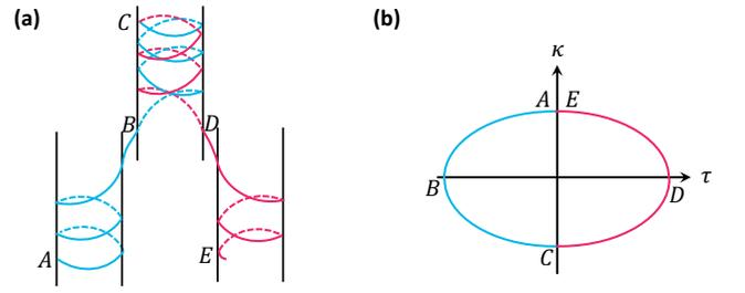
FIG. 2. (a) A winding method of a fiber to obtain non-vanishing Berry's phase for the local coordinate frame (LCF). (b) The path of the LCF in the parameter space. At points  $B$  and  $D$ , the curvature  $\kappa(s)$  of the curve changes sign. At point  $C$ , the sign of the torsion  $\tau(s)$  of the curve flips.
