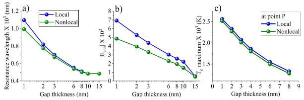
Figure 3. Local and nonlocal calculations of a) absorption resonance wavelengths (computed by Figure 2(a)), b) maximum electric field enhancements, and c) maximum electron temperatures. All these results are plotted versus the nanogap thickness. The induced maximum electron temperature values are calculated at point P depicted in the inset of Figure 2(b).
