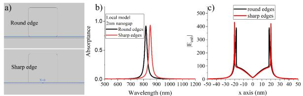
**Figure S3:** a) Round (top panel) and sharp (bottom panel) edge nanostripe geometries in the case of a 2nm nanogap metasurface absorber. The round scenario is the same with the one used in the main paper. b) Absorptance spectrum of the two geometries demonstrated in (a). c) Electric field enhancement computed along the blue line in (a) (bottom of the nanostripe) at each corresponding absorptance resonance: 818nm (round edge) and 852nm (sharp edge).
