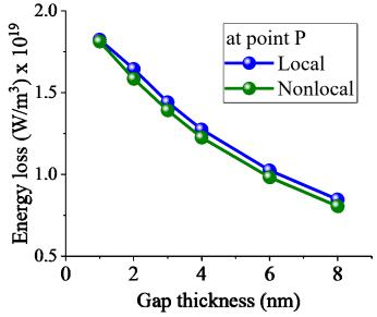
**Figure S5**: Average energy loss delivered to the metallic components of the nanostructure computed at point P shown in Figure 3(c) for a 2nm nanogap metasurface illuminated by a laser intensity of GW/cm<sup>2</sup> in the case of local and nonlocal models.
