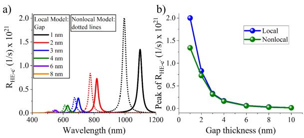
**Figure 4.** a) Generation rate of hot electrons as a function of the wavelength excitation for various nanogap thicknesses computed by the local and nonlocal model. b) The maximum hot electron generation rate at the resonance peaks shown in (a) calculated by local and nonlocal simulations.
