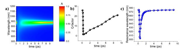
**Figure 7.** a) Tunable ultrafast transient absorption as a function of wavelength and time. b) The computed Q-factor of the absorption resonance response varying in time. c) The tunable absorption resonance wavelength is shifted as a function of time.
