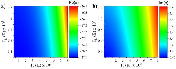
**Figure S6**: (a) Real and (b) imaginary parts of silver permittivity plotted as a function of electron (x-axis) and lattice (y-axis) temperatures. The results are computed under femtosecond laser illumination at the resonance wavelength (818nm) of a 2nm nanogap metasurface.
