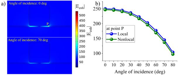
**Figure S4:** a) Computed electric field enhancement distribution by using the local model for normal (top panel) and  $70^{\circ}$  oblique (bottom panel) incident illumination. b) Electric field enhancement as a function of incidence angle for local and nonlocal models computed at point P shown in caption (a). These calculations are for the 2nm nanogap metasurface.
