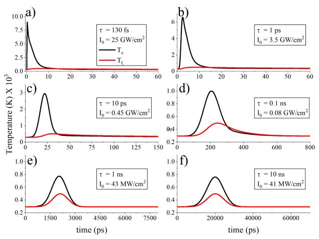
**Figure 5.** Electron (black lines) and lattice (red lines) temperature dynamics for (a), (b) ultrashort femtosecond, (c), (d) picosecond, and (e), (f) slow nanosecond incident pulse durations. All the data are calculated in the point P shown in the inset of Figure 2(b).
