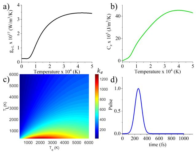
**Figure S1.** a) Electron-lattice coupling factor, b) electron heat capacity, and c) electron thermal conductivity derived from Equation (3). The material characterized by these parameters is silver. d) The envelope of the femtosecond Gaussian pulse with maximum amplitude at  $t = 3\tau$ , where  $\tau = 130 fs$ .
