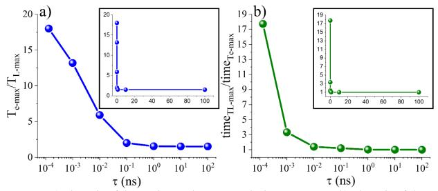
**Figure 6.** a) The ratio of the maximum electron over lattice temperature. b) The ratio of the time when  $T_{e-max}$  occurs over the time when the lattice temperature reaches to  $T_{L-max}$ . Both ratios are plotted in logarithmic scale as a function of the incident pulse duration. These results are calculated from the data presented in Figure 5. The insets show the corresponding plots in linear scale. All the data are calculated in the point P shown in the inset of Figure 2(b).
