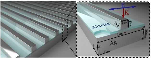
**Figure 1.** Geometry of the gap-plasmon metasurface absorber. Left panel: periodic array of silver nanostripes placed over a silver substrate and an ultrathin dielectric nanogap made of alumina. Inset right panel: unit cell of the gap-plasmon absorber showing the dimensions, materials, and polarization of the incident light.
