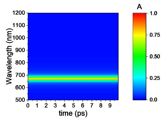
**Figure S9.** Computed absorptance distribution versus time and wavelength obtained by using the temperature varying silver permittivity values defined by Equation 9 in the main paper for 4nm gap thickness plasmonic absorber. Femtosecond ultrafast laser illumination is used with laser input intensity equal to  $I_0 = 5 \ GW/cm^2$ . No temporal change in the absorption spectrum is obtained on vast contrast to Figure 7 in the main paper (2nm gap plasmonic absorber case).
