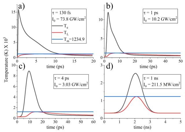
**Figure 8.** Damage (breakdown) study of the presented gap-plasmon metasurfaces. The induced lattice and electron temperatures for a) ultrashort femtosecond, b) one picosecond, c) four picoseconds, and d) slower one nanosecond laser pulse illuminations. The constant blue line depicts the melting temperature of silver.
