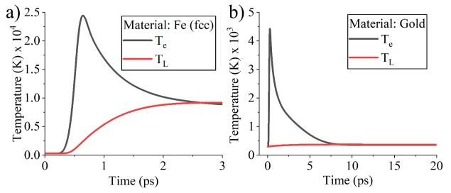
**Figure S2.** Electron and lattice temperatures computed by the current multiphysics simulations and obtained at the surface of a) bulk iron (fcc) and b) 200nm thick flat gold film. The results perfectly agree with previous published works based on analytical approaches.[2,4] All the parameters used in these simulations are identical to the previous analytical works.[2,4]
