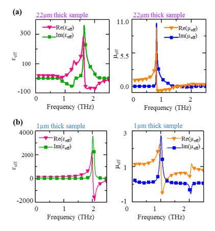
Figure 4. Calculated permeability and permittivity. (a) and (b) Numerically obtained values of effective permeability and permittivity from the S-parameter retrieval method for the 22  $\mu$ m and 1  $\mu$ m samples, respectively.
