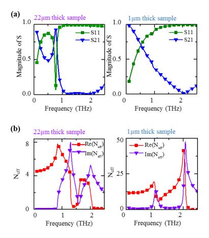
**Figure 3.** Simulated S-parameter and calculated refractive index. (a) Simulated reflection, S11 (green) and transmission, S21 (blue). (b) Calculated complex refractive index of the samples with peak values 7.78+0.96i at 0.839THz and 41.8+22.07i at 2.026 THz for the 22 µm and 1 µm samples, respectively.
