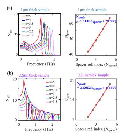
**Figure 8.** Effective refractive index versus substrate refractive index. Calculated effective refractive index for varying the spacer refractive index for (a) 1  $\mu$ m and (b) 22  $\mu$ m thick sample. Change in the peak value of the effective refractive index of the sample w.r.t. the spacer refractive index for (a) 1  $\mu$ m and (b) 22  $\mu$ m thick sample.
