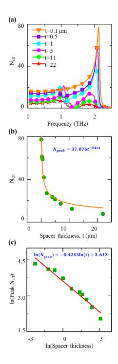
**Figure 6.** Effective refractive index versus substrate thickness. (a) Calculated effective refractive index for the various spacer thicknesses, (b) change in the peak value of the effective refractive index w.r.t. the spacer thickness and (c) natural log of the peak refractive index versus natural log of the spacer thickness.
