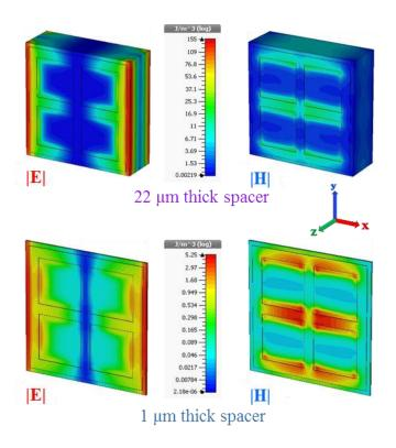
**Figure 5.** Energy density. Simulated distribution of the electric and magnetic energy density at 0.839 THz and 2.026 THz for the 22  $\mu$ m and 1  $\mu$ m samples, respectively.
