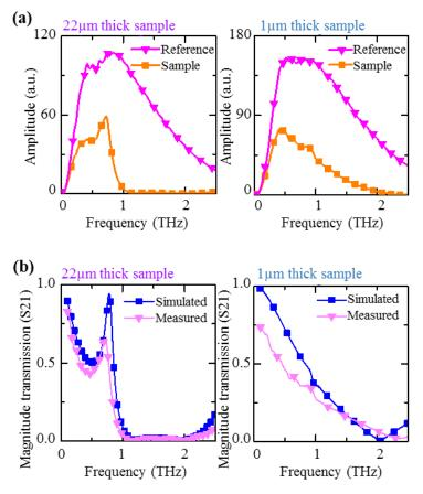
**Figure 2.** Simulated and measured transmission map. (a) Measured transmission amplitude for the 22  $\mu$ m and 1  $\mu$ m thick samples is compared with that of the reference, air and (b) comparison between the simulated and the measured transmission magnitude for the samples is shown for the 22 $\mu$ m and 1  $\mu$ m thick samples, respectively.
