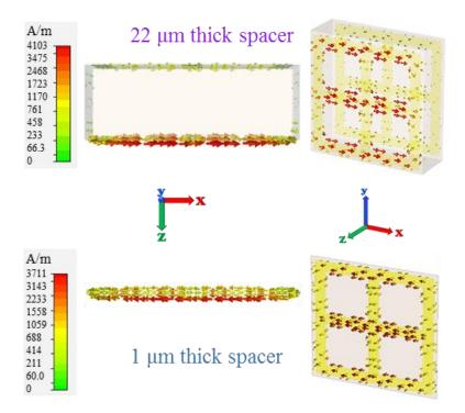
**Figure 7.** Surface current distribution. Top and perspective view of the surface current distribution for normal incident wave along the *z*-direction inside the structure with (a) 22  $\mu$ m thick substrate and (b) 1  $\mu$ m thick substrate.
