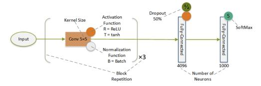
Figure 7: Basic block diagram explanation.
