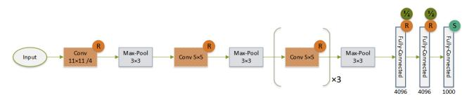
Figure 8: AlexNet architecture.
