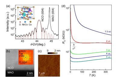
**FIG. 1.** (a) XRD  $\theta$ -2 $\theta$ scan of a 60 uc NCO film on MgAl<sub>2</sub>O<sub>4</sub> (MAO) with a fit to Laue oscillations near the (004) peak (dotted line). Inset: Schematic of NCO crystal structure. (b) HAADF-STEM and (inset) SAED images taken on a 17 uc NCO. (c) AFM topography image of a 5 uc NCO showing atomically flat terraces. (d)  $R_{\Box}(T)$  for 1.5-5 uc films. The dotted line illustrates the twodimensional quantum resistance  $\frac{h}{e^2}$ .
