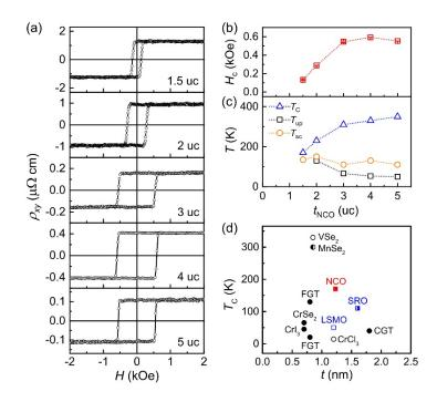
**FIG. 2.** (a)  $\rho_{xy}$  vs H hysteresis at 100 K for 1.5-5 uc NCO. (b-c)  $t_{\text{NCO}}$ -dependence of (b)  $H_c$  at 100 K, and (c)  $T_c$ ,  $T_{\text{up}}$ , and  $T_{\text{sc.}}$  (d)  $T_c$  vs. thickness for epitaxial complex oxide films (squares)<sup>24,25</sup> and 2D vdW magnets (circles).<sup>26-33</sup> Solid symbols: PMA. Open symbols: in-plane magnetic anisotropy.
