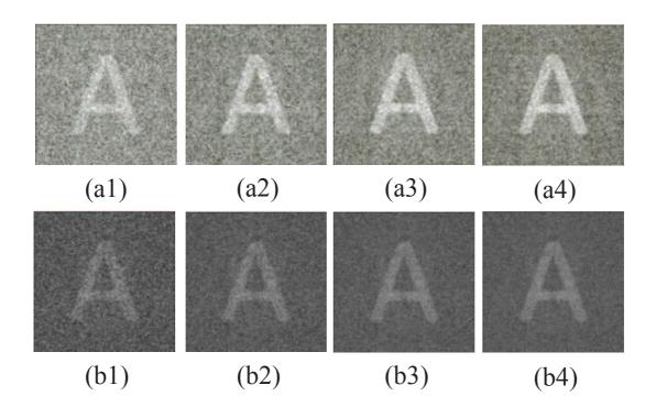
Fig. 3. Top row: the reconstructed images obtained by computational ghost imaging with different measurements. (a1-a4) 1000, 4000, 7000, 10000. Bottom row: the reconstructed images obtained by our method. (b1)m = 500, n = 2, (b1)m = 500, n = 8, (b1)m = 500, n = 14, (b1)m = 500, n = 20.
