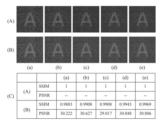
Fig. 6. (A) Images reconstructed by our method without atmospheric turbulence. (B) Images reconstructed by our method with atmospheric turbulence. (a-e) Measurement times of 1000, 2000, 3000, 4000 and 5000, respectively, with m = 500. (C) The SSIM and PSNR values of the images corresponding to the above figures.
