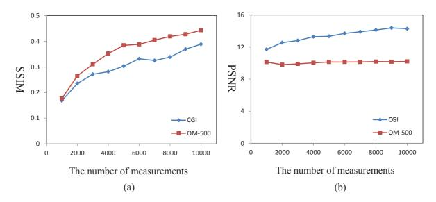
Fig. 4. The (a) SSIM and (b) PSNR curves of the images reconstructed by computational ghost imaging and our method, respectively. CGI: computational ghost imaging, OM-500: our method with m = 500.
