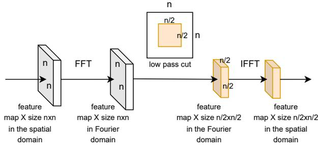
**Fig. 4.** FrequencyLowCut pooling, the proposed, guaranteed alias-free pooling operation. We first transform feature maps into frequency space via FFT, then crop the low frequency components. The result is transformed back into the spatial domain. This corresponds to a sinc-filtered and down-sampled feature map and is fed into the next convolutional layer.
