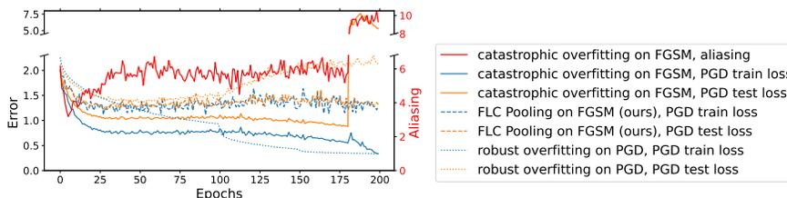
**Fig. 2.** Examples of AT facing catastrophic overfitting and its relationship to aliasing as well as robust overfitting and our FLC pooling. While FGSM training is prone to catastrophic overfitting, PGD training takes much longer and is also prone to robust overfitting. Our method, FLC pooling, is able to train with the fast FGSM training while preventing catastrophic overfitting.
