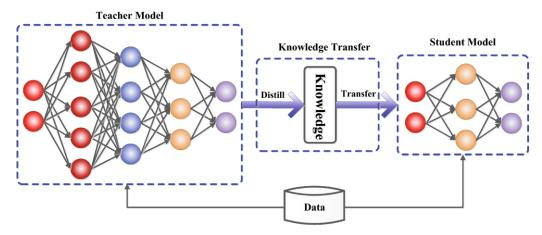
Fig. 2. The general structure of knowledge distillation.
