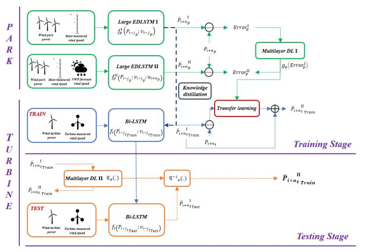
Fig. 4. The proposed KD structure for distilling knowledge from park to turbine.
