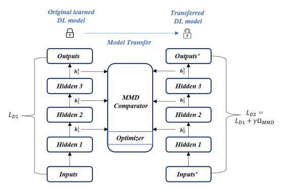
Fig. 1. The architecture of proposed TL with adaptive sparse deep learning
