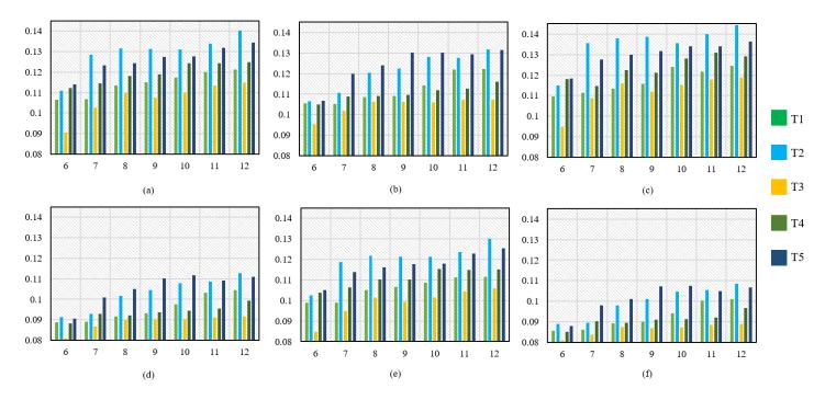
Fig. 6. The multistep RMSE of models with varying prediction algorithms for each turbine: (a) BiLSTM, (b) EDLSTM, (c) KD, (d) EDED-TL, (e) EDBi-TL, (f) KD-TL.
