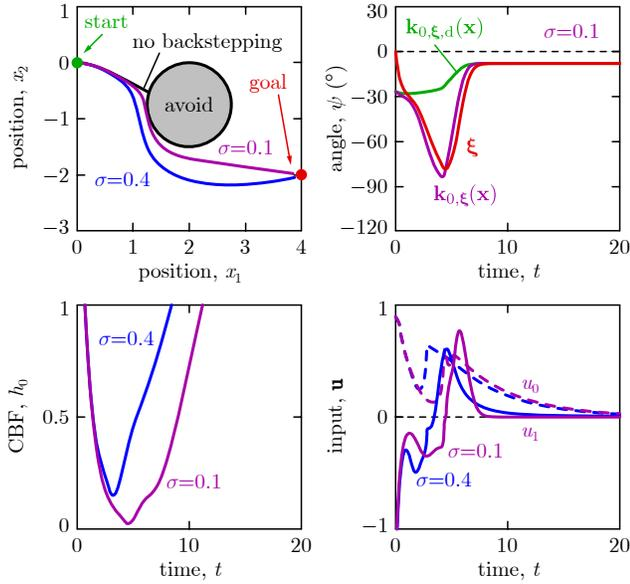
**Fig. 2.** Obstacle avoidance with unicycle model via backstepping. Remarkably, the unicycle is able to drive around the obstacle, while a standard safety filter without backstepping makes the unicycle stop in front of the obstacle.
