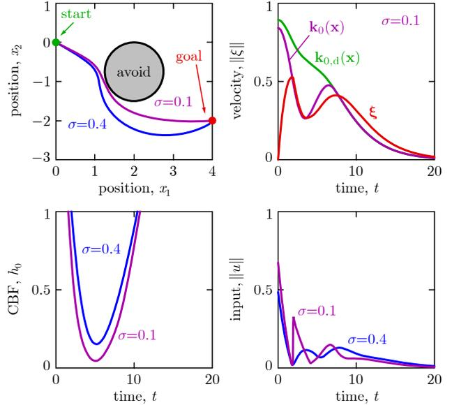
**Fig. 1.** Obstacle avoidance with double integrator model via backstepping. The system successfully avoids the obstacle and reaches the goal, while the conservatism of the route can be tuned by the smoothing parameter.
