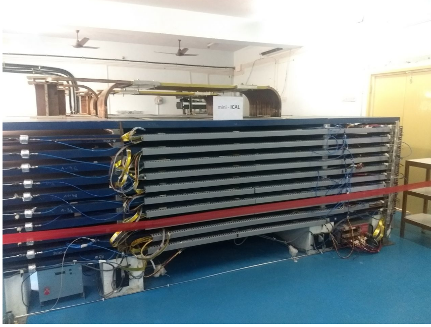
Figure 1. A view of 85 ton miniICAL detector with 10 layers of RPC detector.
