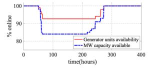
Figure 7. Hourly generator units and active power capacity availability
