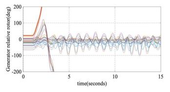
Figure 12. Relative rotor angle of machines at hour 52 without corrective action
