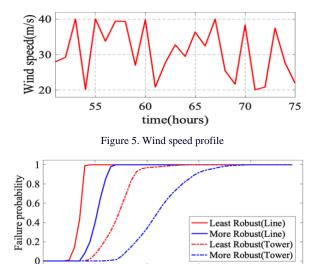
Figure 6. Fragility curve of transmission corridor extracted from [7]
