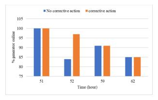
Figure 14. Percentage of the generators online in the two cases of with and without implementing corrective actions
