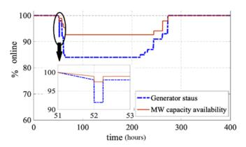
Figure 11. Percentage generators and active power capacity availabilityaggregated model
