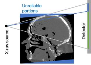
Fig. 2. Illustration for the reliable volume masking. Any ray through an unreliable portion (marked in blue on the image volume) is unreliable and contributes to the mask indicating an unreliable area in a projection (marked in blue on the detector) which should be excluded in the loss calculation for motion estimation.
