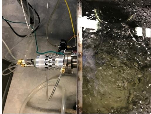
Figure 2: Operation of gliding arc plasmatron in a water tank during PAW production.
