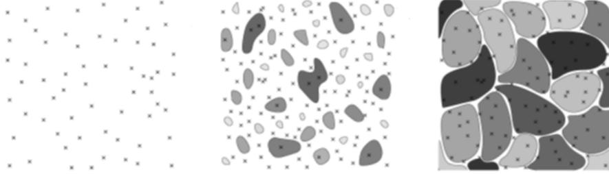
Figure 1: Schematic view of the phase transition from the amorphous (left) to fully-crystalline (right) state (from [11]).
