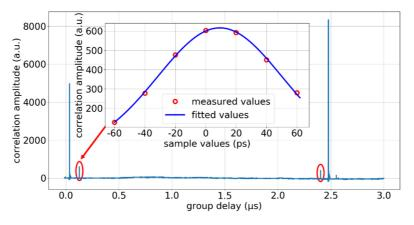
Fig. 2. Correlation function over time shows four reflections: two introduced reflections and two reflections from glass to air transition. Inset: pulse approximation of one reflection peak.
