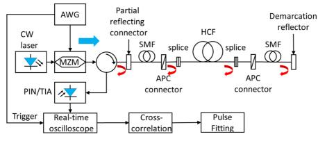
Fig. 1. Measurement setup of the C-OTDR to determine the group delay of two NANF- HCF.
