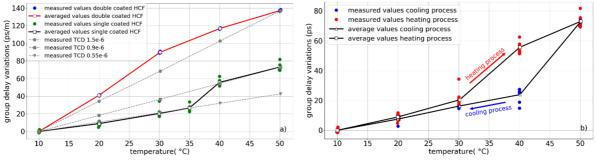
Fig. 3 a) Measured group delay variations as function of temperature with measured TCD as linear fit, b) Measured group delay variations of the single coated HCF during heating and cooling process which shows a hysteresis.
