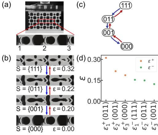
FIG. 2. Robust pathways in sample A. (a) Sketch of the sample with three defects labeled 1, 2 and 3 respectively. (b) Snapshots of the defect beams during a compression/decompression cycle, showing the distinct states. (c) The transition graph of the sample A. (d) The switching fields  $\epsilon^\pm$  A ordered from large to small.
