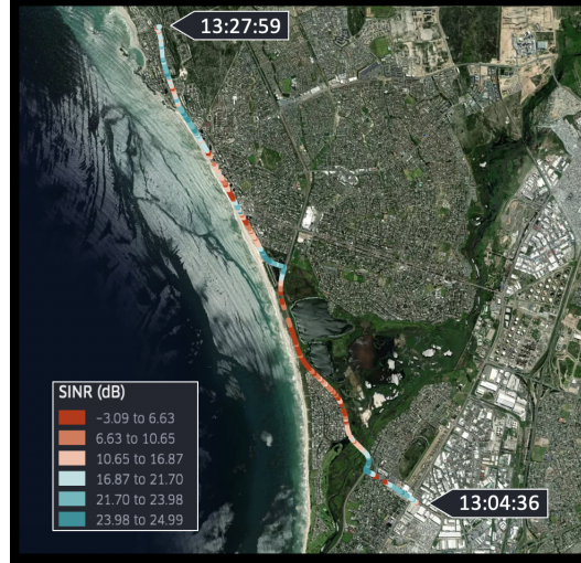
Figure 7: Location of the drive test with the captured SINR measurements. Note the changes in signal-to-noise power as the user equipment moves through certain areas.
