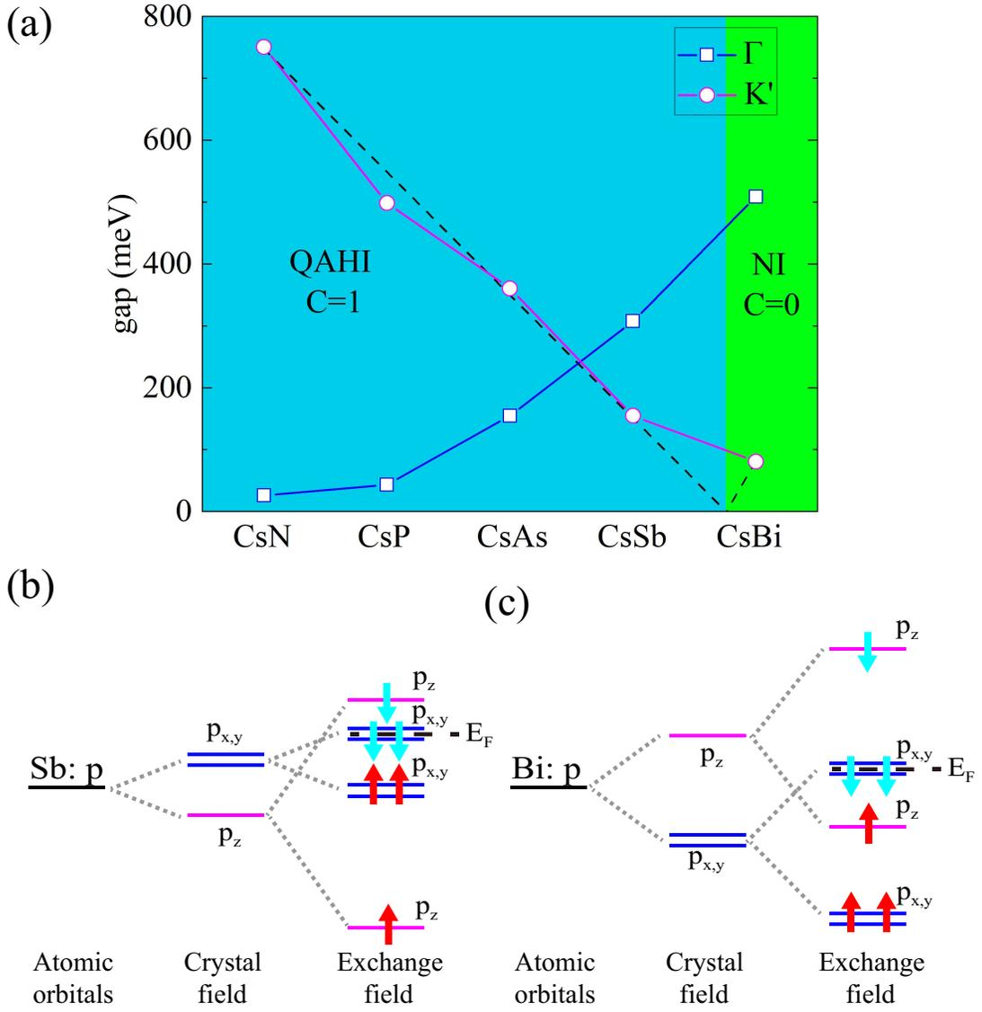
FIG. 7. (a) The gap of CsY ( $Y = \text{N, P, As, Sb, Bi}$ ) at  $\Gamma$  and  $K'$  points. The dotted line is the fitting  $K'$  point gap variation trend. (b, c) The schematic illustration of energy level for Sb-p orbital in CsSb (b) and Bi-p orbital in CsBi (c).
