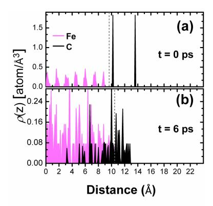
Figure S2. Calculated density profiles  $\rho(z)$  of dissolution process of the graphite layers in molten Fe are presented. (a) and (b) correspond to the structures at the beginning and the conclusion of the simulation. The dashed line marks the interface defined as the highest z coordinate of the Fe atoms.
