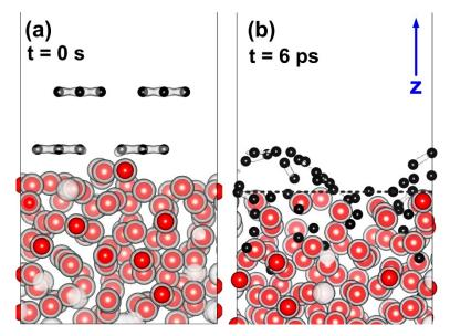
Figure S1. The decomposition and dissolution of the graphite sheets in molten iron at T = 1823 K (~ 1550 °C). The red and black balls represent Fe and C atoms respectively. The gray shade surrounding the atoms represents electronic charge density around each atom which also indicates the atomic bonds. In (b) one can see the disappearance of C–C bonds as the graphite sheets are dissolved in molten Fe.
