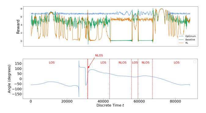
Fig. 8 – Beam selection results for a BS serving a UAV comparing RL versus a simple baseline algorithm. The optimal result (best beam pair) is also included. The top plot presents the reward is the magnitude of the equivalent channel for the i-th beam pair at the time t (higher reward values are better). The bottom plot shows the AoA  $\theta$  at the UAV at each time t.
