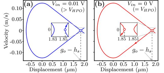
Fig. 6. Analysis of pull-out using phase-portrait. Pull-out does not occur for input greater than the pull-out voltage,  $V_{HPO}$ , as displacement  $g_o - h_s$  lies on the open trajectory. Pull-out occurs when input equals  $V_{HPO} = 0$  V as  $g_o - h_s$  lies on the closed trajectory.
