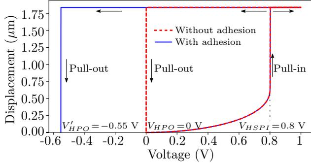
Fig. 4. Numerical simulation of the static characteristics of the hybrid actuator without (red dashed) and with (blue solid) adhesion forces. Due to adhesion, the pull-out voltage is reduced from  $V_{HPO} = 0$  V to  $V'_{HPO} = -0.55$  V. However, the static pull-in voltage ( $= 0.8$  V) remains unchanged.
