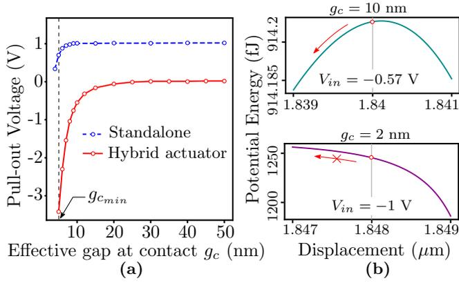
Fig. 8. (a) Variation in the pull-out voltage with respect to the change in the effective gap at contact  $g_c$ . As effective gap increases, the pull-out voltage tends towards the electrostatically estimated (without adhesion) value. (b) Energy-displacement plots for  $g_c = 10$  nm and 2 nm. The presence of an energy barrier prevents pull-out for  $g_c = 2$  nm ( $< g_{c_{min}}$ ). Note that the  $\circ$  represents  $(g_o - h_s - g_c)$  in both cases.
