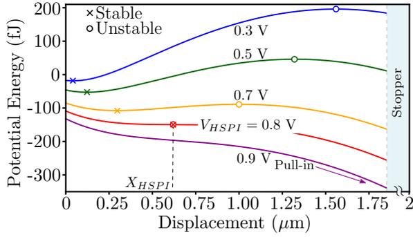
Fig. 3. Potential energy-displacement plot depicting static pull-in. Stable and unstable equilibrium displacements coincide at static pull-in voltage,  $V_{HSPI} = 0.8$  V, with travel range  $X_{HSPI} = 0.62$   $\mu\text{m}$ .
