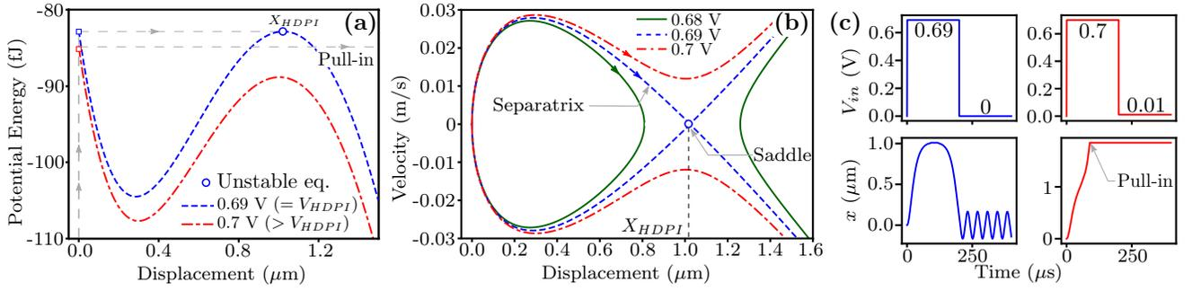
Fig. 5. Analysis of dynamic pull-in using (a) Potential energy-displacement plot. Initial energy at  $x = 0$  equals the energy at the point of unstable equilibrium when the step input equals the dynamic pull-in voltage,  $V_{HDPI} = 0.69$  V. Any step input greater than  $V_{HDPI}$  results in dynamic pull-in. (b) Phase-portrait. The trajectory becomes open when dynamic pull-in occurs. (c) Numerical simulation based on Ref. [20].
