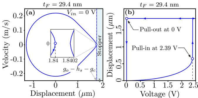
Fig. 9. (a) Phase-portrait depicting that the pull-out voltage, in the presence of adhesion, is 0 V, achieved with a reduced ferroelectric thickness of  $t_F = 29.4$  nm. (b) Numerical simulation of the static characteristics of the hybrid actuator with  $t_F = 29.4$  nm.
