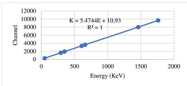
**Figure 4.** Energy calibration results showing the correlation between energy and spectrometric channel numbers
