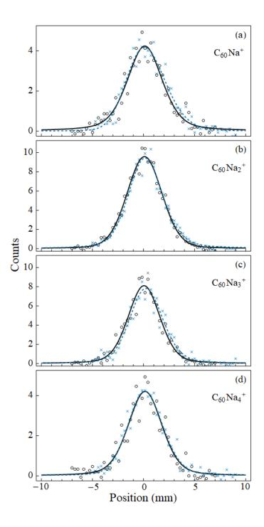
**Fig. 2** Beam deflection measurements for  $C_{60}Na_{n=1-4}$ . Circles (crosses) denote data points with the electric field turned off (on). The counting rates of selected ions in the strongly collimated beam were on the order of a few per second. The solid lines are symmetric pseudo-Voigt<sup>31</sup> fits to the "field-off" profile , while the dashed lines are asymmetric pseudo-Voigt fits to the "field-on" profile. In all cases the beam deflection is negligible.
