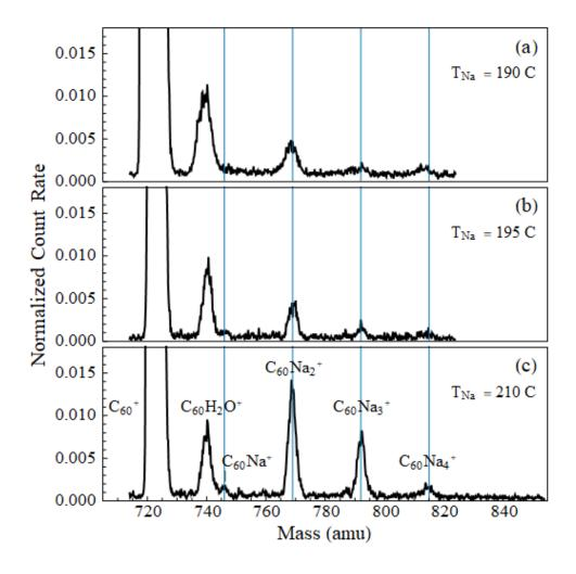
**Fig. 1** Mass spectra of  $C_{60}Na_n^+$  complexes with the corresponding Na pick-up cell temperatures indicated. All spectra are normalized to the intensity of the  $C_{60}^+$  peak. The  $C_{60}Na^+$  signal is weak for all temperatures. Panels (a) and (b) show the conditions used for deflection measurements of the  $C_{60}Na_2^+$  and  $C_{60}Na_3^+$  peaks, respectively, while (c) gives the conditions for  $C_{60}Na^+$  and  $C_{60}Na_4^+$  deflections.
