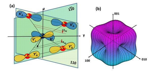
**Figure 2.** (a) VB states  $X_{\nu}$  and  $Y_{\nu}$  near BZ center using basis rotated by 45 degrees around z axis.  $X_{C}(Y_{C})$  state makes strong covalent  $\sigma$  bond only with  $X_{A}(Y_{A})$  state above (below) it. (b) absolute value of permanent dipole of VB HH and LH states versus direction of k-vector.
