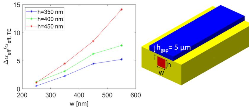
Fig. 8. Scanning  $w$  and  $h$  in 3D FDTD for  $h_{\text{gap}} = 5 \text{ nm}$  ( $\text{SiO}_2$ ),  $T_{\text{metal}} = 0.5 \mu\text{m}$ , and  $L = 5.5 \mu\text{m}$  at 1550 nm. This scan is performed to know if the results are like the results in 2D represented in Fig. 4(a).
