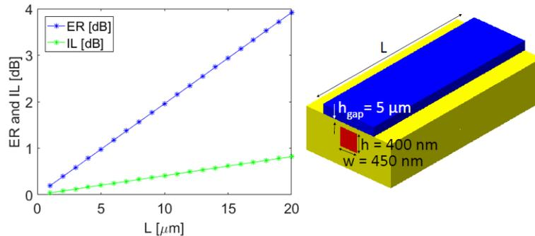
Fig. 5. Estimated polarization extinction ratio and insertion loss of a TE-pass polarizer with continues metal which consists of an HPW of length  $L$ . The dimensions of the HPW are  $w = 450$  nm,  $h = 400$  nm and  $h_{\text{gap}} = 5$  nm ( $\text{SiO}_2$ ). The wavelength is 1550 nm.
