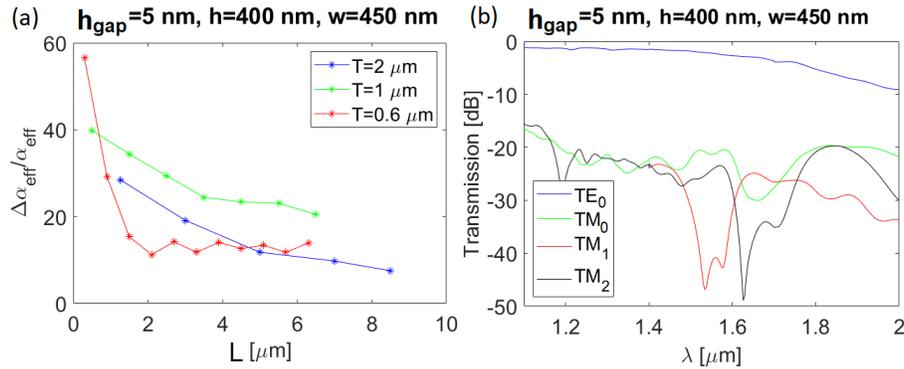
Fig. 6. Estimation of the  $FoM = PER/IL$  of the TE-pass polarizer with a segmented metal of  $T_{\text{metal}}$  (a) The wavelength is fixed to 1550 nm and the HPW have the optimized values. In (b) the spectrum of the TE-pass polarizer with  $L = 5.5 \mu\text{m}$  and  $T_{\text{metal}} = 0.5 \mu\text{m}$ .
