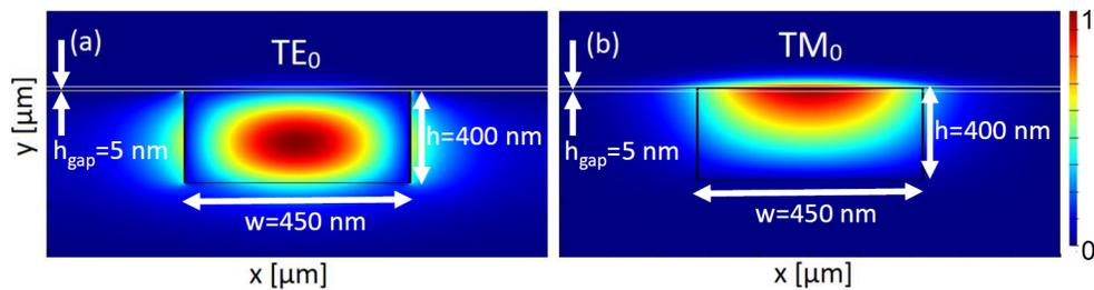
Fig. 1. Example of an electric field of the  $\text{TE}_0$  (a) and  $\text{TM}_0$  mode (b) in an HPW. The slot is made of  $\text{SiO}_2$ . The  $\text{TE}_0$  mode is concentrated in the Si core while the  $\text{TM}_0$  mode is concentrated in the slot and the interface between the metal and the slot. The wavelength is 1550 nm.
