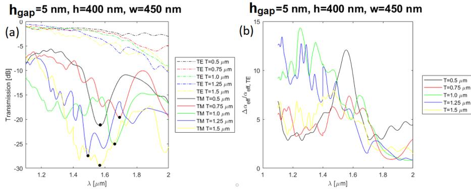
Fig. 12. Scanning the period  $T$  of the optimized plasmonic TE-pass polarizer. In (a) the transmission of the TE and TM modes and in (b) the  $FoM = \Delta\alpha_{eff}/\alpha_{eff,TE}$ . The dots in Fig. 12(a) are the points selected to study the grating behavior.
