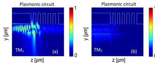
Fig. 7. Filtering of TM<sub>1</sub> (a) and TM<sub>2</sub> (b) for the optimized TE-pass polarizer with  $w = 450 \text{ nm}$ ,  $h = 400 \text{ nm}$ ,  $h_{\text{gap}} = 5 \text{ nm}$  (SiO<sub>2</sub>),  $T_{\text{metal}} = 0.5 \mu\text{m}$ , and  $L = 5.5 \mu\text{m}$  for 1550 nm.
