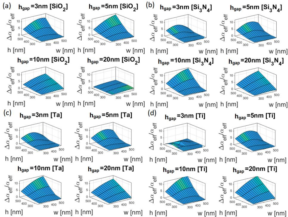
Fig. 4. Study of the  $\text{FoM} = \Delta\alpha_{\text{eff}}/\alpha_{\text{eff, TE}}$  for the different parameters of the HPW  $w$ ,  $h$  and  $h_{\text{gap}}$  with a  $\text{SiO}_2$  (a),  $\text{Si}_3\text{N}_4$  (b), Ta (c) and Ti (d). Typical parameters for  $w$ ,  $h$  and  $h_{\text{gap}}$  are used.
