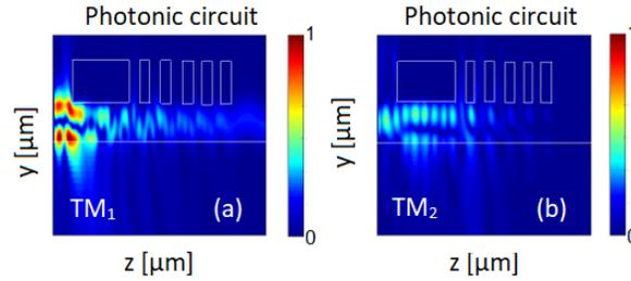
Fig. 11. Optimized TE-pass polarizer with segmented metal for a photonic circuit for TM<sub>1</sub> (a) and TM<sub>2</sub> (b) at 1550 nm.
