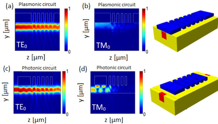
Fig. 3. The electric field of the  $TE_0$  mode passing through the TE-pass polarizer (a) in a plasmonic circuit. In (b), the electric field of the  $TM_0$  mode being filtered by the TE-pass polarizer. In (c), there is the electric field of the  $TE_0$  mode passing the TE-pass polarizer while in (d) the  $TM_0$  mode is filtered. The wavelength is 1550 nm.
