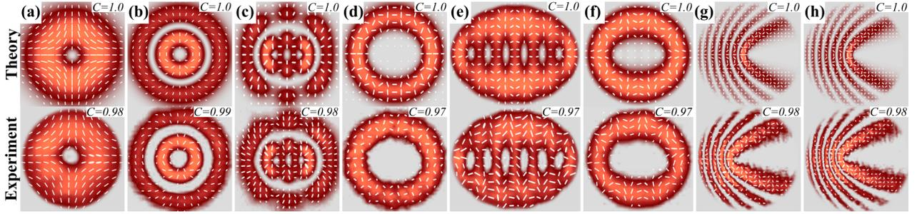
**Figure 5.** Transverse polarisation overlapped with the corresponding intensity profile of exemplary vector modes generated in various coordinate systems. (a)-(b)  $\mathbf{U}_{LG}^{\ell,p}$ ; (c)-(d)  $\mathbf{U}_{IG^h}^{p,m,\varepsilon}$ ; (e)-(f)  $\mathbf{U}_{MG^h}^{m,\varepsilon}$ , and (f)-(g) parabolic-Gauss vector modes. The specific parameters for each case are detailed in the main text.
