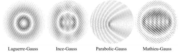
**Figure 1.** Example of the binary holograms encoded on a DMD to generate, from left to right, the modes  $LG_0^1$ ,  $IG_3^3$ ,  $PG$  and  $MG_6^6$
