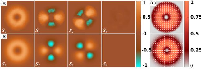
**Figure 3.** Experimental (a) and theoretical (b) Stokes parameters  $S_0$ ,  $S_1$ ,  $S_2$  and  $S_3$  used to reconstruct the polarisation distribution of the vector mode  $U_{LG}^{1,0}$ , with  $(\theta, \alpha) = (\pi/4, 0)$  shown in (c).
