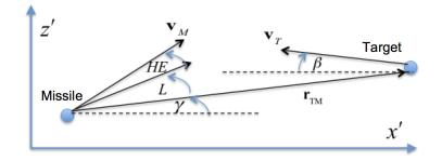
Fig. 2 Planar Heading Error
