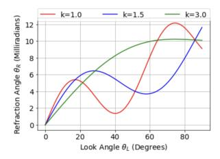
Fig. 4 Radome Refraction Angle as Function of Look Angle
