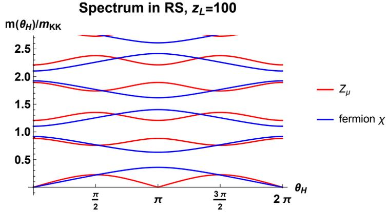
Figure 1: The mass spectrum of gauge fields  $Z_\mu^{(n)}$  and fermion fields  $\chi^{(n)}$  (type 1A) in the RS warped space is displayed. The warp factor is  $z_L = 100$  and the bulk mass parameter of  $\Psi$  is  $c = 0.25$ . There is no level crossing in the spectrum.
