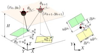
Fig. 2. Reachable spaces for the left (green) and right (yellow) feet, defined with bounds relative to the frame  $\{x_c, y_c, z_c\}$  attached at the COM. Left and right rectangles are symmetric about the  $x_c$  axis when  $u^{\theta} = 0$ .
