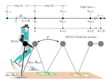
Fig. 7. MPC implementation on Digit. The MPC is solved at time  $\xi$  during step (k-1)th step. Its solution  $u_k$  becomes available at  $\xi + \delta t$  and is used to update the swing foot configuration at touchdown. Red dots on the continuous time t axis are the times when the LIP state,  $x_{init}$  is extracted from the Digit to predict  $x_k$  as required by the MPC. This prediction is based on the solution (1)-(2) of the continuous dynamics of the LIP.
