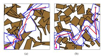
Fig. 4. Example environments and paths generated by the MPC. (a) Polygonal obstacles. (b) Rotated rectangular obstacles.
