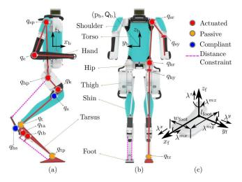
Fig. 5. The bipedal robot Digit and relevant coordinates. (a) Side view; the kinematic loops actuating the tarsus and foot are highlighted with the dotted magenta lines. (b) Back view. (c) Ground contact constraints.
