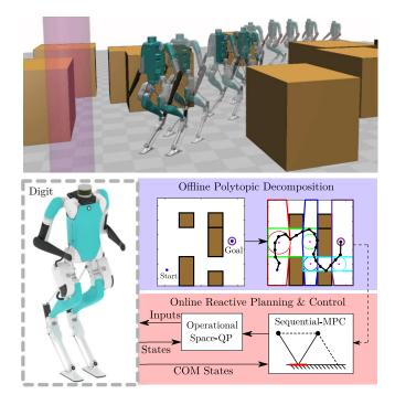
Fig. 1. Top: The bipedal robot Digit navigating amidst obstacles. Bottom: Overview of the proposed framework. An RRT-guided sequential decomposition of the workspace to obstacle-free polytopes is used to formulate a sequence of MPC programs that drive the LIP to the goal position and avoid collisions with static and moving obstacles. The suggested LIP-based plan is then realized on Digit using a QP-based operational space controller.
