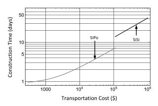
**Figure 11.** Construction time of the least expensive system for the baseline economic scenario but varying the transportation cost.
