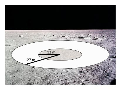
**Figure 1.** Landing pad configuration with inner and outer zone dimensions used in this study. (Lunar surface image credit: NASA)
