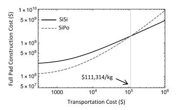
**Figure 9.** Cost of SiSi and SiPo for the baseline economic scenario but varying the transportation cost.
