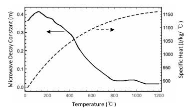
**Figure A-3.** Microwave decay constant and specific heat used to model microwave sintering of lunar soil.
