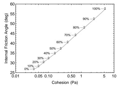
**Figure A-1.** Parametric plot of friction and cohesion as functions of relative density (annotated circles on plot) for a lunar simulant, following Heiken et al. [81] which follows Mitchell et al. [82,83].
