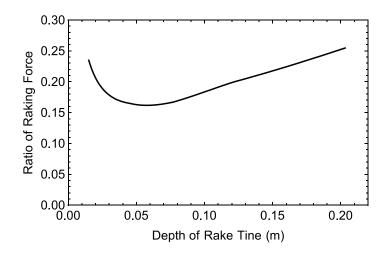
**Figure A-2**. Ratio of raking force in lunar soil to terrestrial farm soil versus depth or rake in the soil, calculated by the Balovenev equation.
