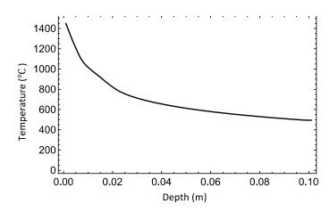
**Figure A-4.** Model's predicted temperature profile after microwaving 200 kW/m<sup>2</sup> at 2.45 GHz into lunar soil for 5.34 minutes. The average temperature is above the sintering temperature in the top 1 cm, but we assume thermal conductivity (otherwise neglected in this model) averages the temperatures over that length scale.
