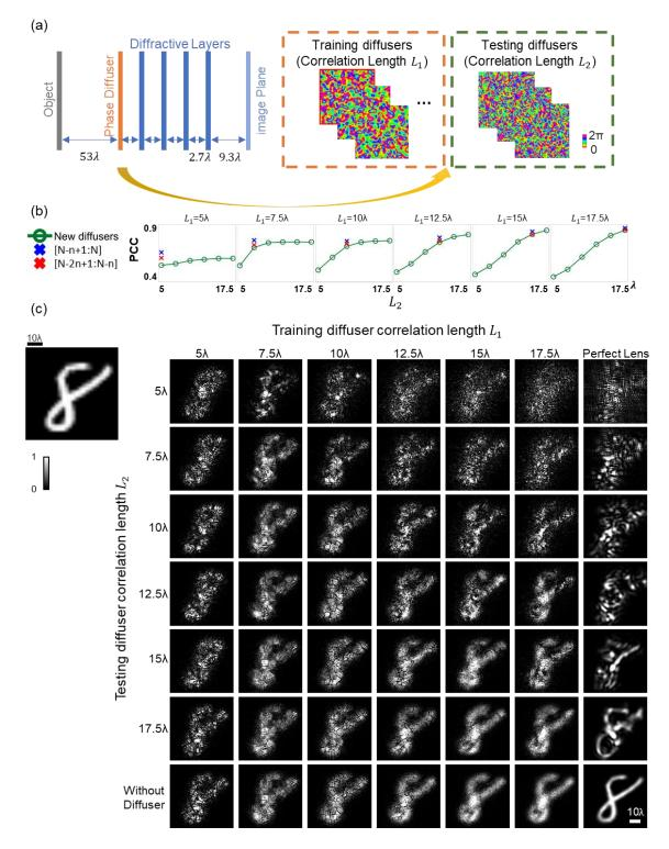
Figure 2. Imaging through random diffusers with different correlation lengths. (a)Training and design schematic of a 4-layered diffractive optical network seeing through new, random phase diffusers. (b) PCC values of diffractive neural networks trained with  $L_I=5\lambda$ , 7.5 $\lambda$ , 10 $\lambda$ , 12.5 $\lambda$ , 15 $\lambda$ ,
