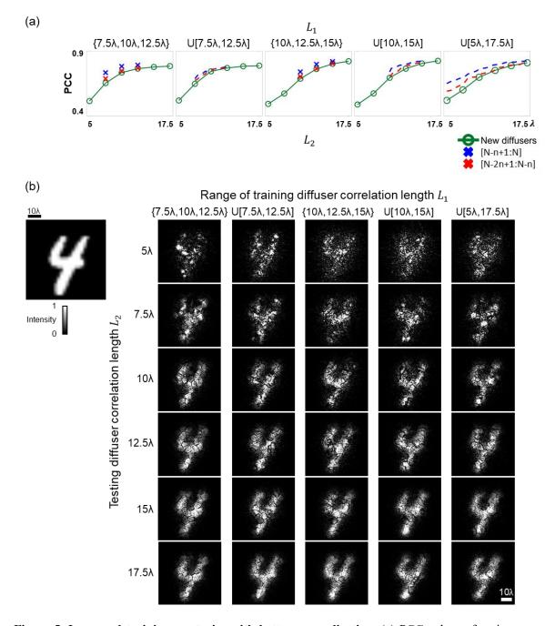
Figure 5. Improved training strategies with better generalization. (a) PCC values of various diffractive neural networks trained and tested with different  $L_1$ ,  $L_2$  combinations. (b) Example images seen through new random diffusers using the diffractive networks in (a). The contrast of the images was enhanced for visualization (see the Methods section for details).
