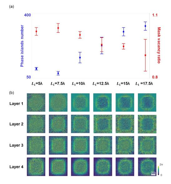
Figure 4. Quantification of the circular phase islands within the diffractive layers. (a) The number of the phase islands and the mask vacancy ratio of the diffractive layers trained with different random phase diffusers ( $L_1 = 5\lambda$ , 7.5 $\lambda$ , 10 $\lambda$ , 12.5 $\lambda$ , 15 $\lambda$  and 17.5). (b) Corresponding diffractive layer phase profiles of the converged diffractive networks.
