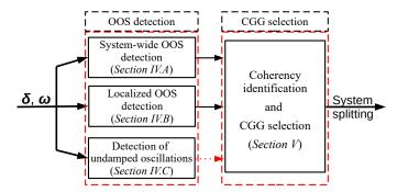
Fig. 1: High-level overview of the controlled splitting scheme
