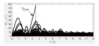
Fig. 13: Branch angle differences for splitting transients after fault on line 21–22
