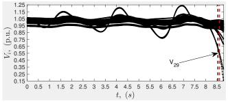
Fig. 16: Bus voltage magnitudes after tripping of line 28-29
