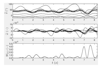
Fig. 4: Undamped oscillation after disconnecting of line 28–29
