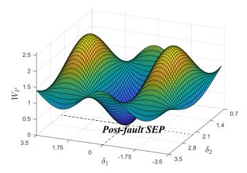
Fig. 2: Concept of post-fault SEP in potential energy well
