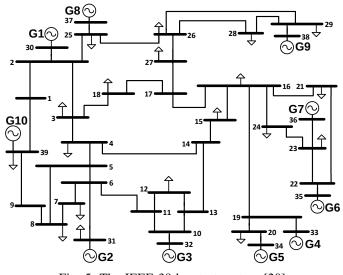
Fig. 5: The IEEE 39-bus test system [20]
