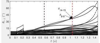
Fig. 7: Branch angle differences for fault on line 16-17
