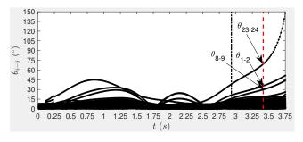
Fig. 10: Branch angle differences for fault on line 21–22
