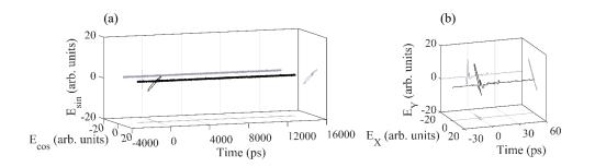
Fig. 3. Three-dimensional plot of the retrieved terahertz E-field vector waveform (a) before and (b) after the evaluation of the angle  $\phi$ . In (b), only the data around the peak structure is plotted. The retrieved polarization is consistent with the angle of the transmission axis of WGP2 ( $\beta = -50^{\circ} \pm 180^{\circ}$ ).
