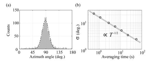
Fig. 5. (a) Statistical distribution of the frequency-averaged azimuth angles derived from the 1800 data segments of length  $80/\Delta f$ . (b) Standard deviation of  $\sigma$  as a function of the averaging time *T*. The gray line shows a  $T^{-1/2}$  dependence.
