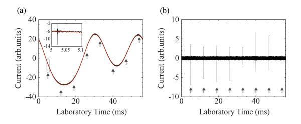
Fig. 2. (a) Current signal recorded on channel 0 after averaging (black line). The integration time for averaging was about 5 minutes. The red curve is the result of the fit for the baseline subtraction. The arrows indicate the times when sharp spikes appear in the signal. (Inset: Magnification of the data around the first spike at  $\tau \approx 5$  ms). (b) The "flattened" signal (after the baseline subtraction).
