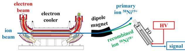
FIG. 3. Sketch of the experimental arrangement at the CSRm electron cooler. The scintillation particle-detector was appropriately placed behind the dipole magnet downstream of the electron cooler for stopping and counting the recombined ions.
