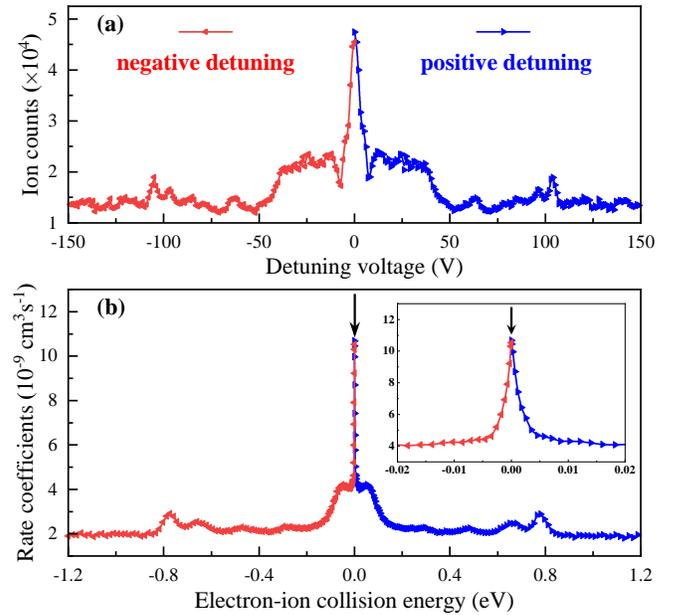
FIG. 4. (a) The original recorded recombined ion counts for detuning voltages up to  $\pm 150$  V. (b) The derived rate coefficients for the corresponding electron-ion collision energies ranging from  $-1.2$  eV to  $+1.2$  eV. The negative sign refers to collision energies that result from negative detuning voltages. The inset highlights the recombination rate-coefficient near zero electron-ion collision energy.
