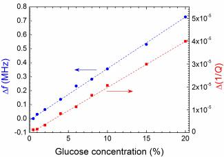
Fig. 4. Resonance frequency shift (circles) and changes in inverse *Q*-factors (squares) dependencies on concentration of glucose in aqueous solution.
