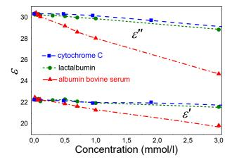
Fig. 7. Real and imaginary parts of permittivity dependencies on concentration of albumin bovine serum (triangles and dash-dot line), lactalbumin (circles and short-dashed line) and cytochrome C (squares and dashed line) in aqueous solutions.
