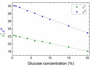
Fig. 6. Real (squares) and imaginary (circles) parts of permittivity dependencies on concentration of glucose in aqueous solutions.
