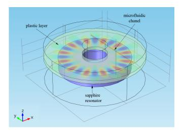
Fig. 2. Numerical geometric model for simulation of the measurement cell and axial component of electric field distribution.
