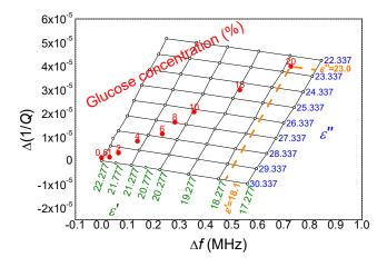
Fig. 5. Nomogram chart. Calculated net for the resonant frequency shift and changes in the inverse quality factor for a microfluidic channel filled with substances with varying real and imaginary parts of the permittivity (see text for details). Red points show the experimentally obtained data for resonant frequency shift and changes in inverse *Q*-factor as functions of glucose concentration in water solution.
