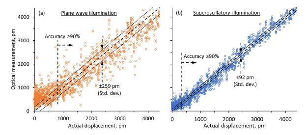
**Fig. 2. Optical measurements of nanowire displacement.** Optically measured versus actual values of nanowire displacement for (a) plane wave and (b) topologically structured superoscillatory illumination. Dotted lines above and below the ideal correlation diagonals are plotted at ±1 standard deviation. Dashed vertical lines denote minimum nanowire displacements that can be measured with accuracy exceeding 90% (relative error <10%).
