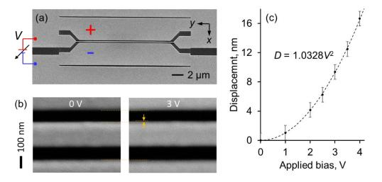
**Fig. S1. Nanowire position calibration**. (a) SEM image of the entire nanowire sample, showing the electrode configuration for electrostatic control of [x direction] position; (b) representative pair of high magnification images of the (y direction) midpoint of the nanowire from which the dependence of nanowire displacement on applied bias – panel (c) – is derived.
