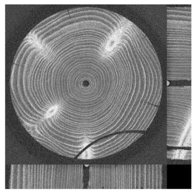
Figure 3. The tomographic data can be virtually cut in any direction. The figure contains the three orthogonal cuts through the center of mass of the cylindrical wooden block.
