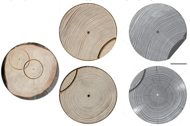
Figure 2. For the tomographic imaging using X rays, two cylinders with a diameter of 180 mm each were prepared, see photographs. The related tomography slices near the surface are represented on the right. The length bar corresponds to 50 mm.
