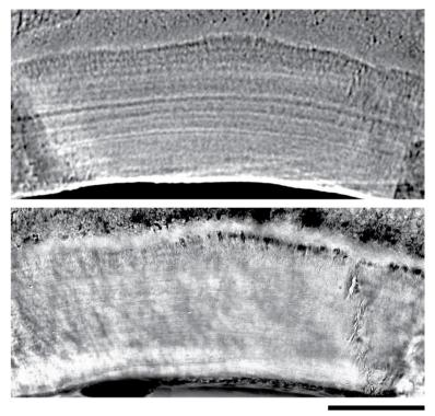
Figure 7. Comparison of incremental layer appearance for same region using hard X-ray tomography (top image) and optical imaging (bottom image). The length bar corresponds to  $100 \mu m$ .
