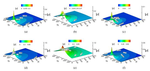
Figure 3: Distributions of  $|\rho|$  associated with different transmission conditions. a) Condition (19), or (25), Case 1. b) Condition (27), Case 1. c) Condition (30), Case 1. d) Condition (19), or (25), Case 2. e) Condition (27), Case 2. f) Condition (30), Case 2.
